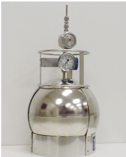
An evacuated air testing canister. The pressure inside the canister is initially set lower than the indoor air, causing air to flow into the canister when the valve is opened.
