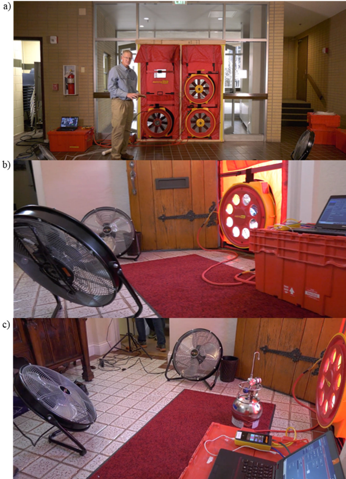
Figure 5. Photos from an industrial multi-blower (panel a) and residential single blower door (panels b and c) CPM test deployment.
