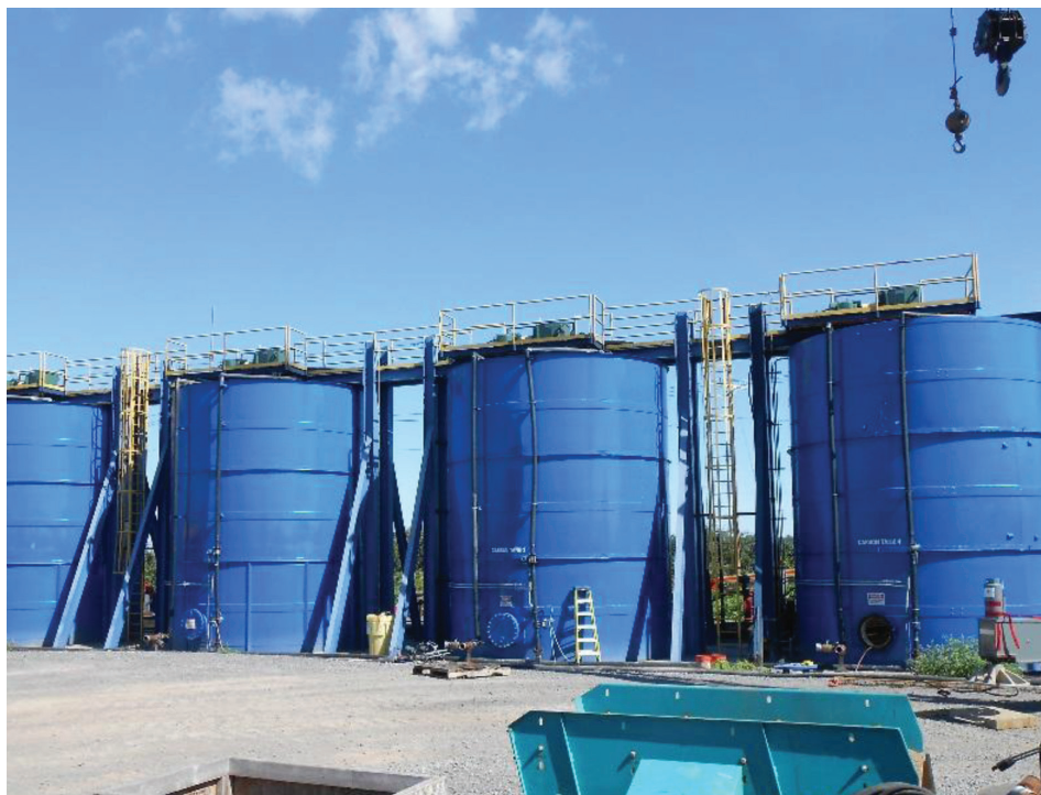
FIGURE 9 Sand/AC slurry mixing tanks.
