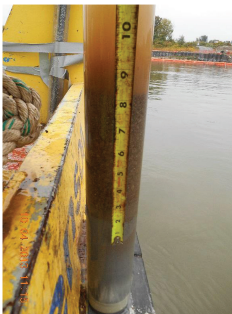
FIGURE 11 Core sample showing verification of cap layer thickness.
