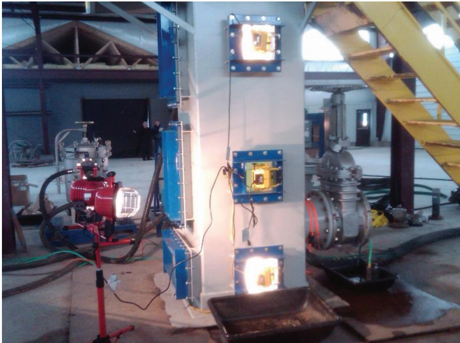
FIGURE 8 Laboratory physical model evaluation of cap and amendment settling velocities and layer consistency post placement.
