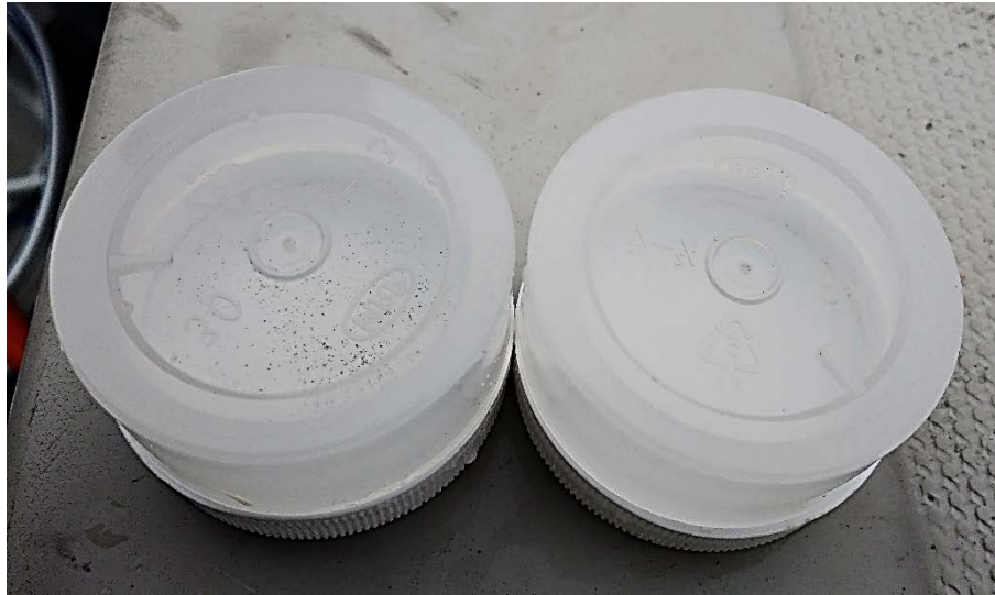
Figure 14: Contaminated peeper with particles (left) vs peeper without any contamination (right).
