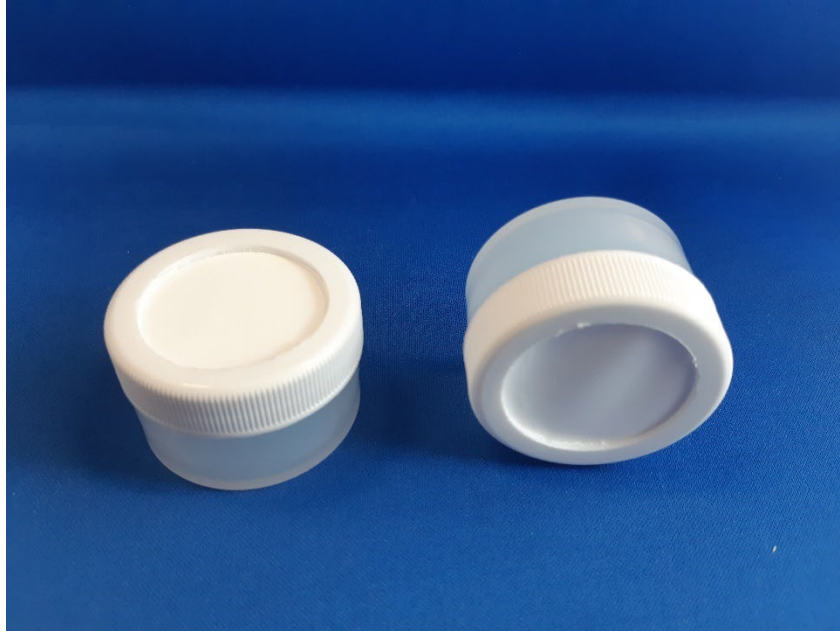
Figure 2-1: Photographs of the peeper design selected for the laboratory experiment and field demonstration (SiREM), showing the peeper vial and membrane surface. The peeper vial contains 15 mL of peeper water.
