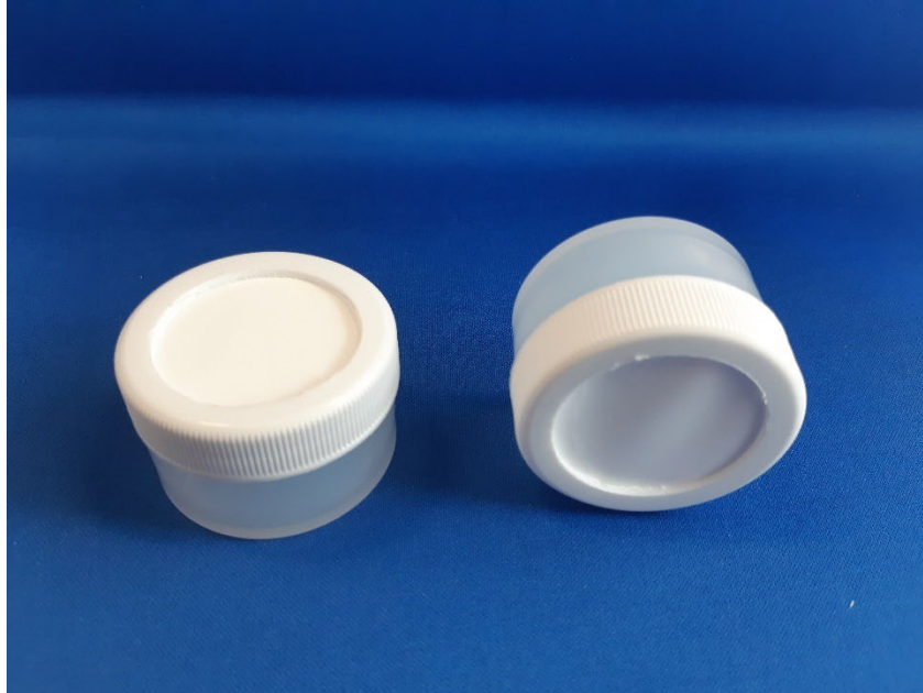
Figure 2-1: Photographs of the peeper design selected for the laboratory experiment and field demonstration (SiREM Laboratories), showing the peeper vial and membrane surface. The peeper vial contains 15 milliliters (mL) of peeper water.
