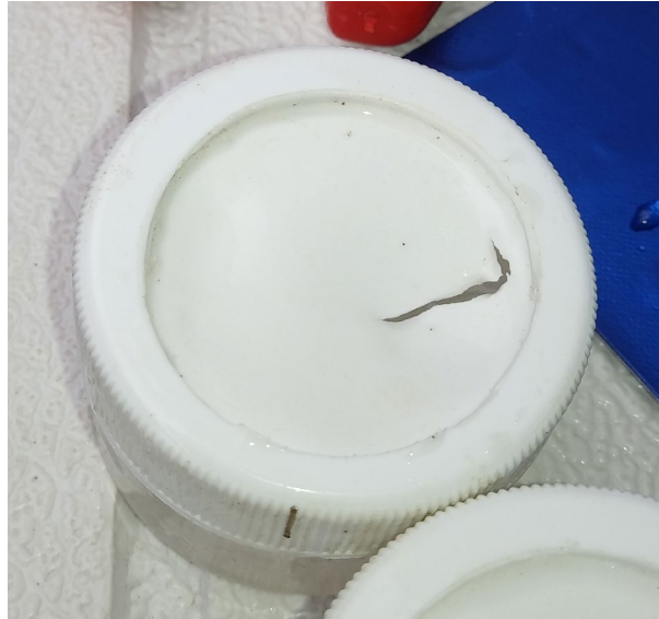
Figure 2-19: A damaged peeper (torn peeper membrane).
