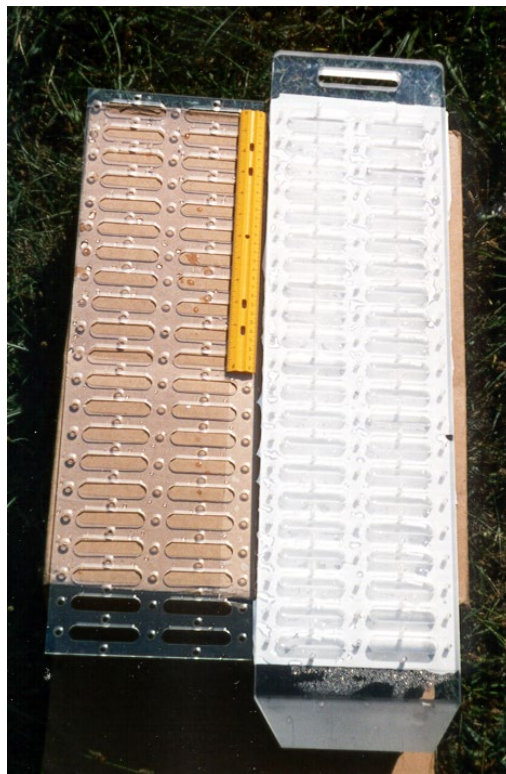
Figure 1-1: General Hesslein (1976) Peeper design (42 peeper chambers), from the United States Geological Survey ( https://www.usgs.gov/media/images/peeper-samplers ).
