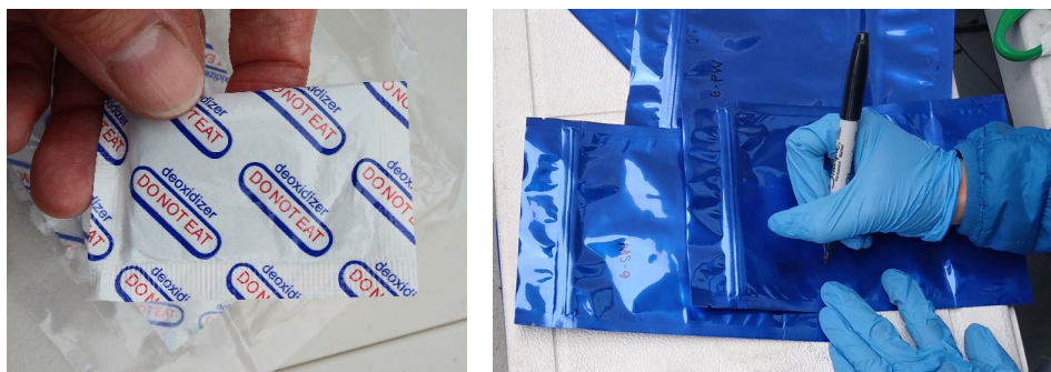
Figure 2-18: A “500-cc” oxygen absorbent “oxy muncher” packet (left) and blue zipseal bags for storing peepers (right).
