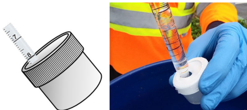
Figure 2-8: Peeper water extraction using a serological pipette.
