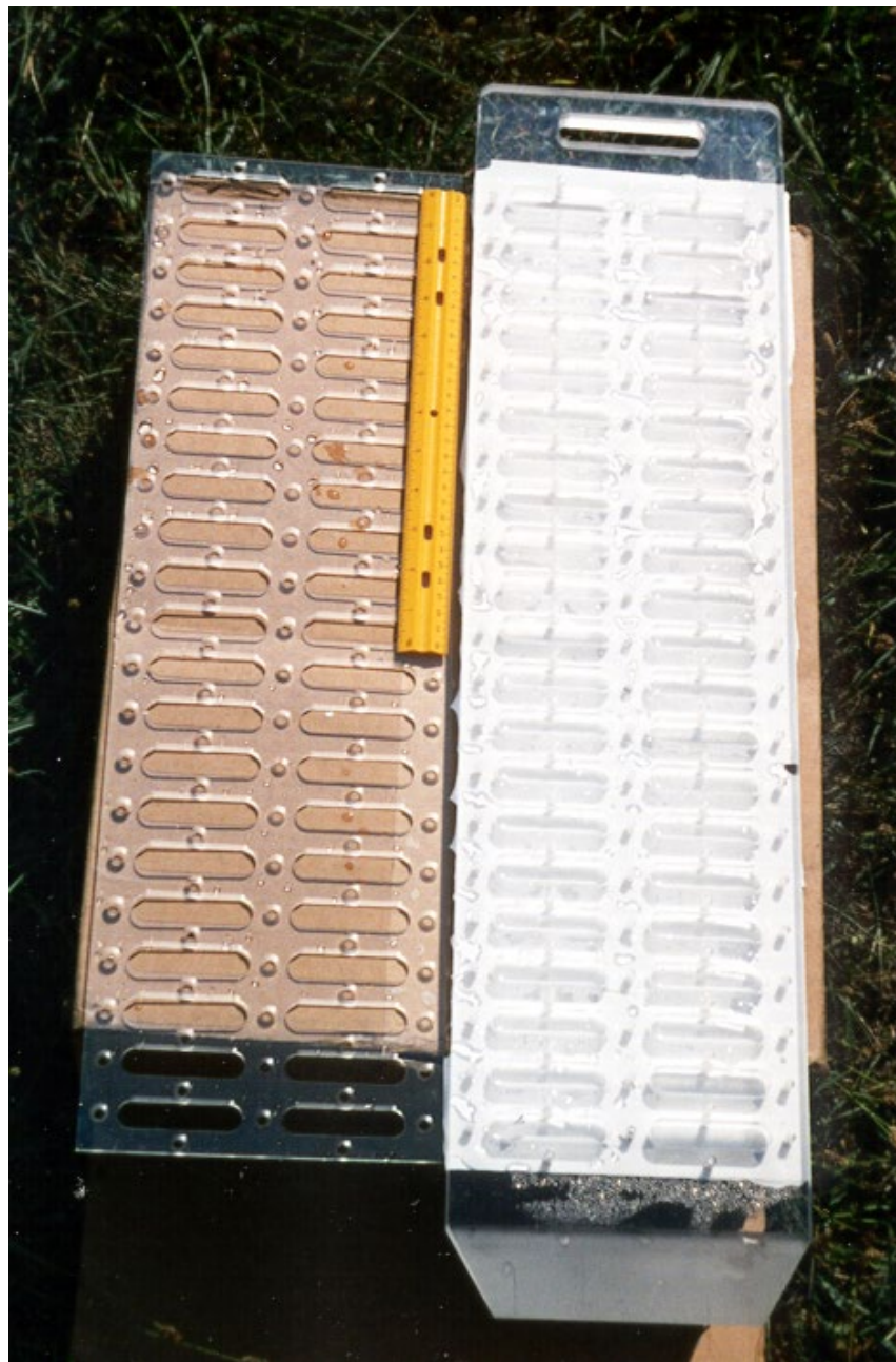
Figure 3. General Hesslein (1976) peeper design (42 peeper chambers), from USGS ( https://www.usgs.gov/media/images/peeper-samplers ).
