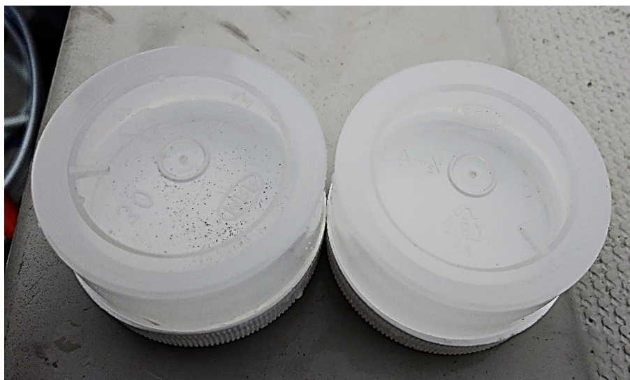
Figure 2-22: Contaminated peeper with particles (left) versus a peeper without any visible particle contamination (right).
