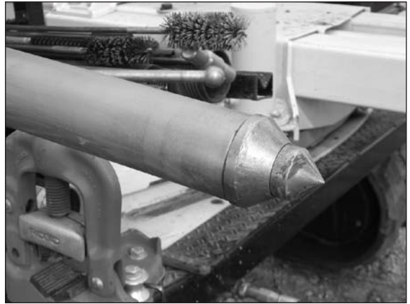
Figure 4.21. Thread the cutting shoe and point onto the sample tube.
