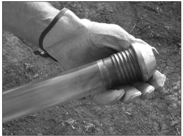
Figure 4.7. Place either end of the liner onto the extended shank cutting shoe. (This is used in place of a spacer ring or core catcher)
