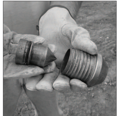
Figure 4.11. The MC5 Closed Piston Point slides into the cutting shoe.
