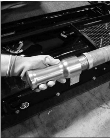
Figure 4.24. Place drive cap onto sampler drive head.
