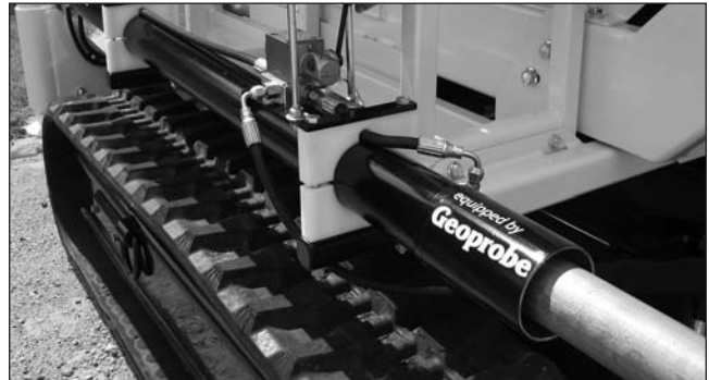
Figure 4.30. The Hydraulic Liner Extruder helps remove the liner.
