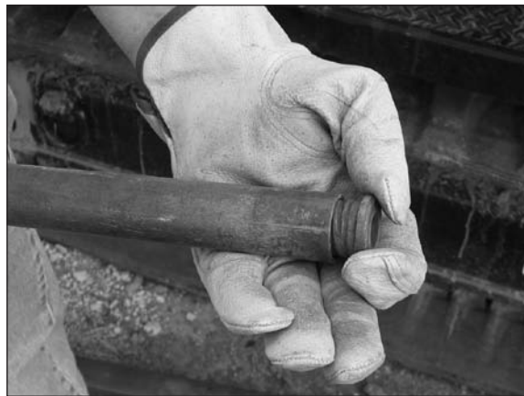
Figure 4.22. The MC5 Plug is threaded onto the end of the 1.25-inch light-weight center rod.
