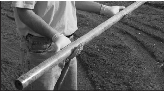
Figure 4.31. MC5 Liner filled with soil core.
