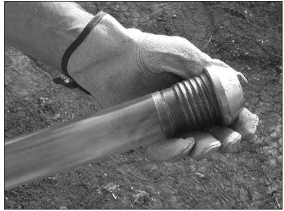
Figure 4.19. Place either end of the liner onto the extended shank cutting shoe. (This is used in place of a spacer ring or core catcher)
