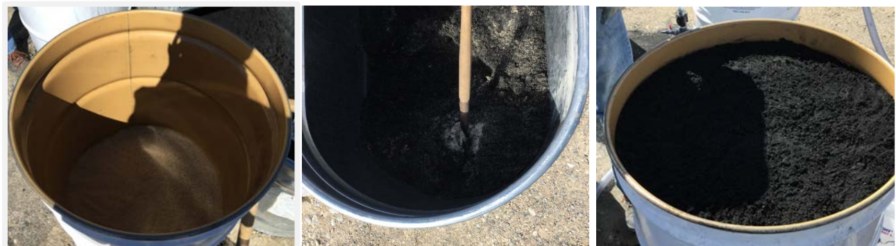
Figure 5. Rembind™ media mixed with sand.
