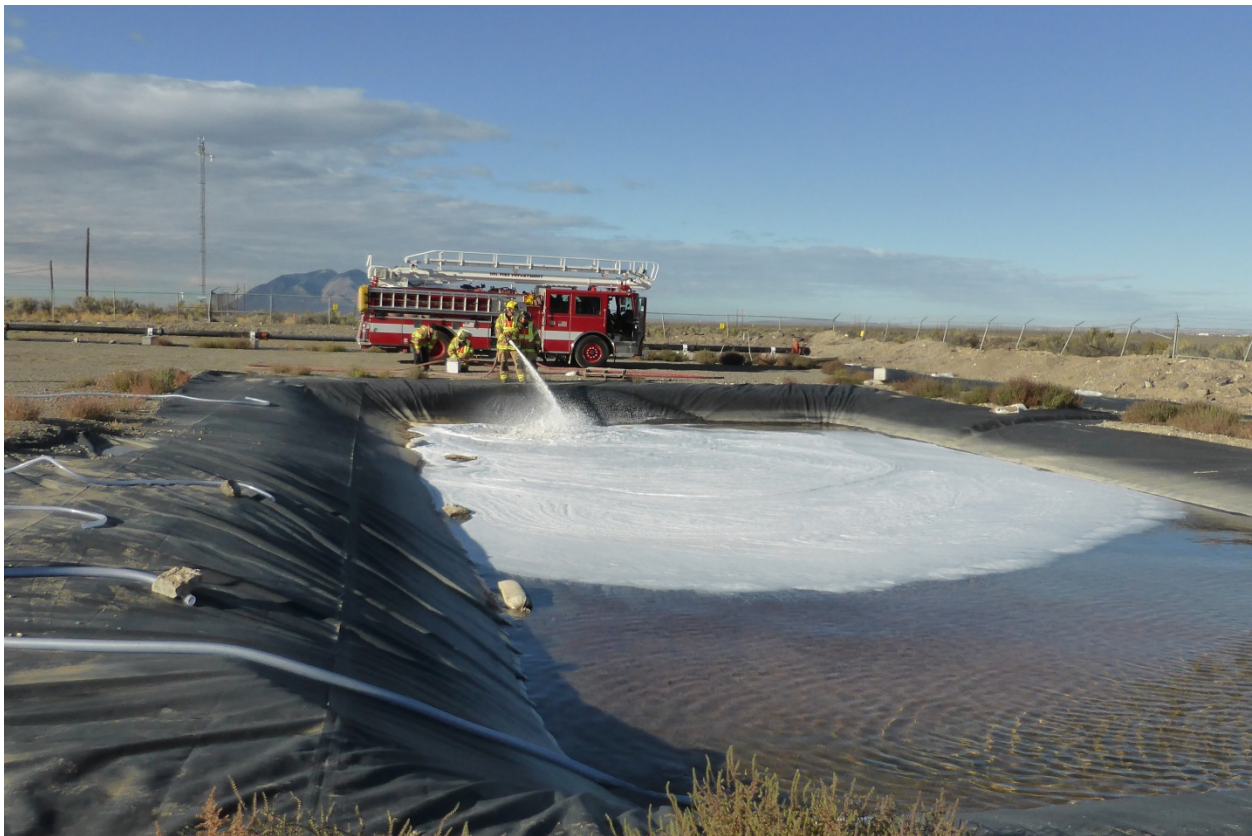
Figure 7. AFFF sprayed to contaminate lagoon water.
