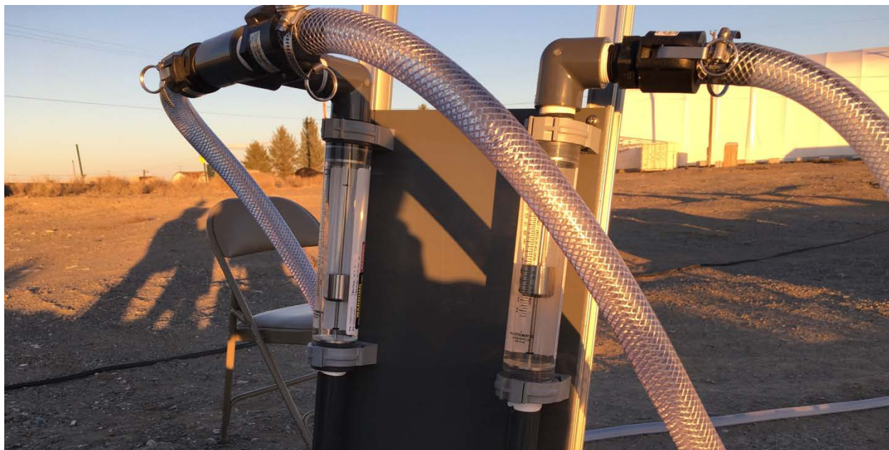
Figure 10. Inlet flow control during testing.
